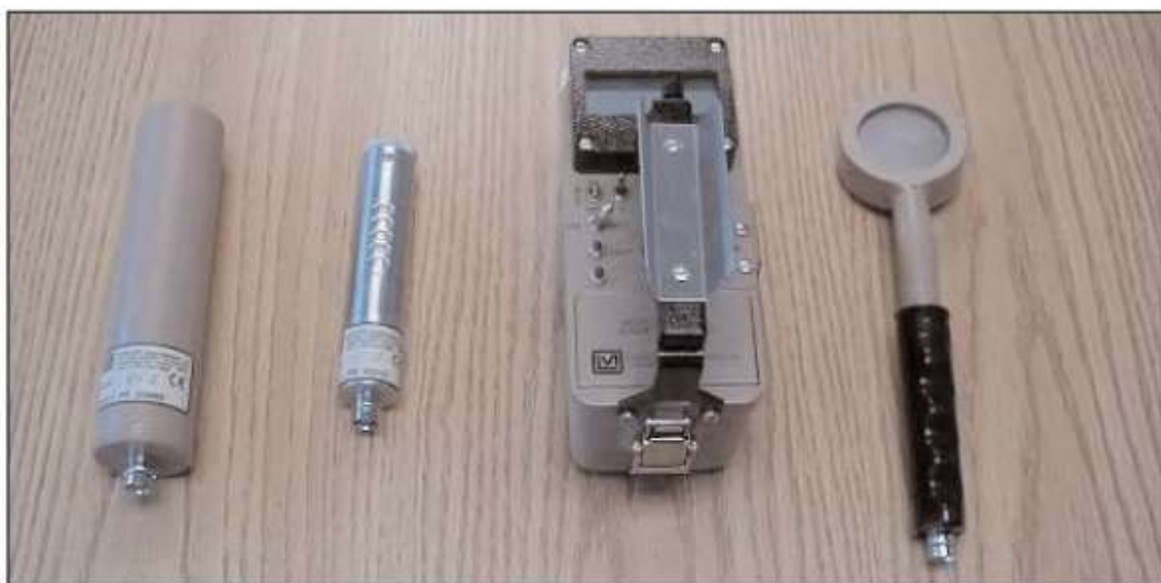
Ludlum Response Kit (left to right): Gamma Scintillator probe, energy-compensated G-M probe, survey meter, G-M pancake probe
