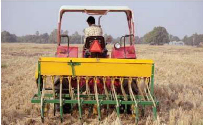
A tractor-drawn ZT seed-cum-fertilizer drill
