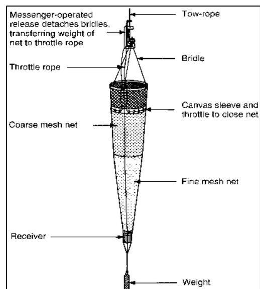
The determination of the volume of water filtered through any plankton net is essential for the estimation.
