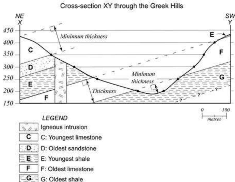
*Completed geological cross-section*
