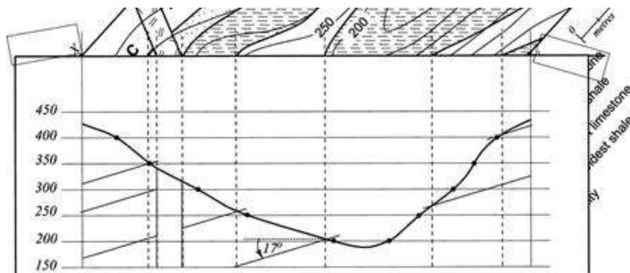
*Drawing a geological cross-section*
