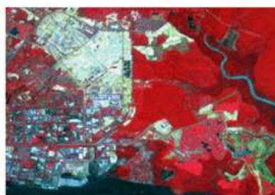
False colour composite multispectral SPOT image: Red: XS3; Green: XS2; Blue: XS1
