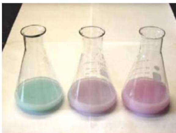
Figure 2 Same colour changes for magnesium chloride back-titration as in Figure 1, but for cloudy (opaque) sample solution, eg milk. Left flask: blue colour well before endpoint. Centre flask: last trace of blue/purple. Right flask: pink/red colour at endpoint
